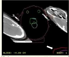
Fig. 3. A Vendor submission viewed with the RRT. This submission has several parameters with incorrect values. The incorrect parameters include (at least) the number of columns in the CT scan, the X offset of the dose array, and the Y offset of the dose array. (Dose is only visible in the lower right corner of the display).
