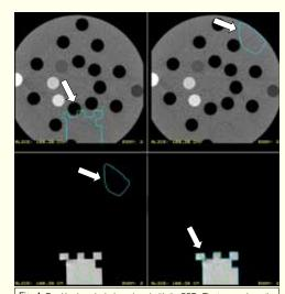
Fig. 4. Two Vendor submissions viewed with the RRT. The two panels on the left are from one submission; the two on the right are from a second submission the next day after the vendor corrected a problem in the Z coordinates of the dose array. Green represents a "structure" and cyan represents an isodose line. The two top panels are at the same Z offset while the two bottom panels are at a different Z offset.
